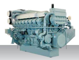
16-cylinder, 4-stroke, water-cooled diesel engine, with direct-injection, turbocharger, air-cooler, built-up heat exchanger and sea water pump.
