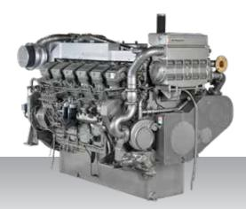
12-cylinder, 4-stroke, water-cooled diesel engine, with direct-injection, turbocharger, air-cooler, built-up heat exchanger and sea water pump.
